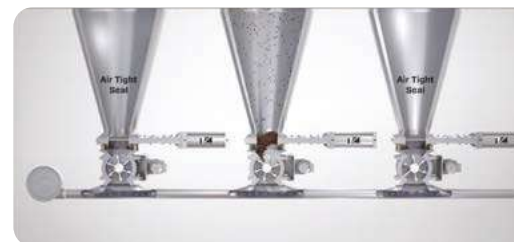
Enhance conveying efficiency by preventing air loss
