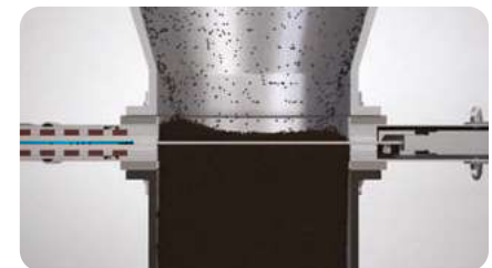
Displacement area as an alternative to packing materials into an end seal
